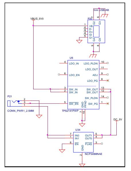
Figure 21. Input Power Section
