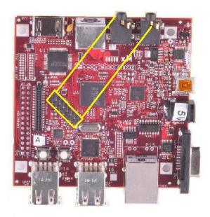
Figure 72. JTAG Cable Placement
