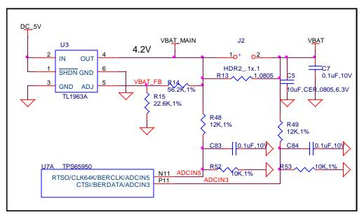
Figure 23. Processor Current Measurement
