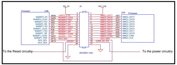
Figure 51. Main Expansion Header Processor Connections
