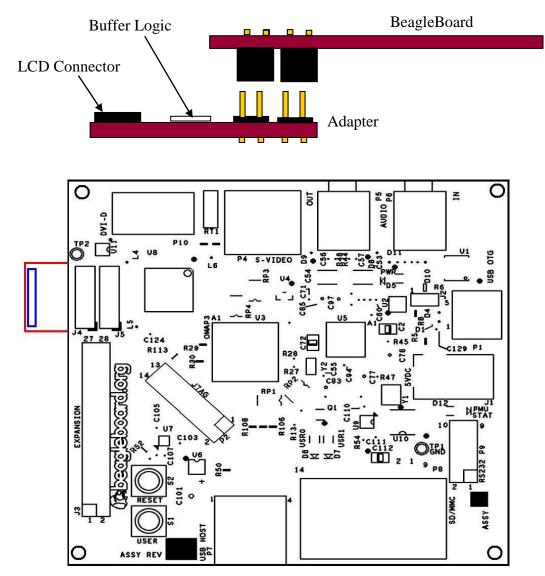
Figure 65. Bottom Mount LCD Adapter
