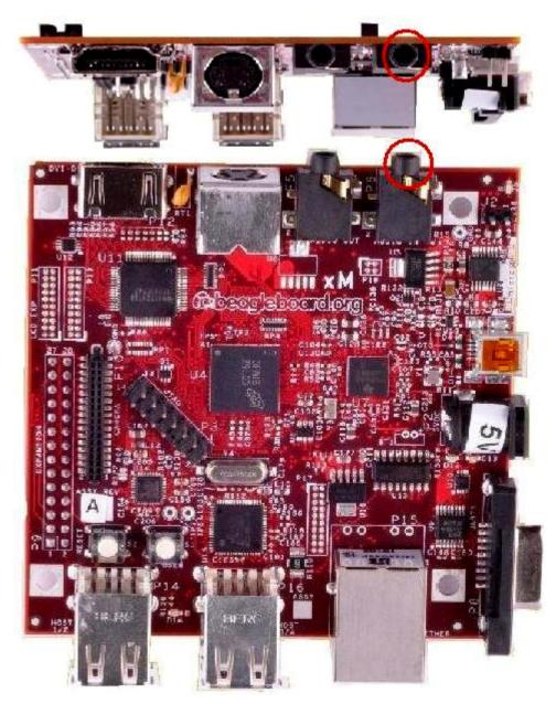
Figure 13. BeagleBoard Audio In Cable Connection
