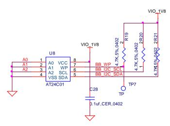
Figure 83. BeagleBoard Expansion Board EEPROM Schematic
