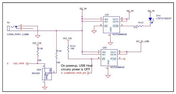
Figure 20. Overvoltage Protection
