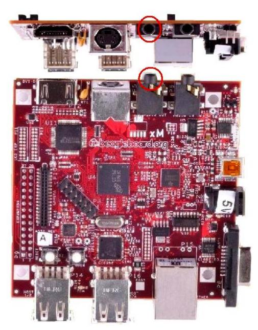
Figure 12. BeagleBoard Audio Out Cable Connection
