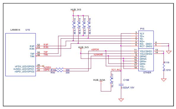
Figure 41. USB Based Ethernet Design
