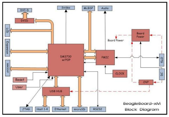
Figure 18. BeagleBoard-xM High Level Block Diagram
