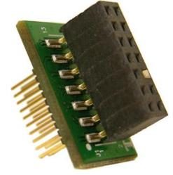
Figure 71. JTAG 14 to 20 Pin Adapter
